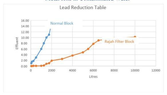
Flow Diagram of Lead reduction of Normal Block and Rajah Filter Blocks.
